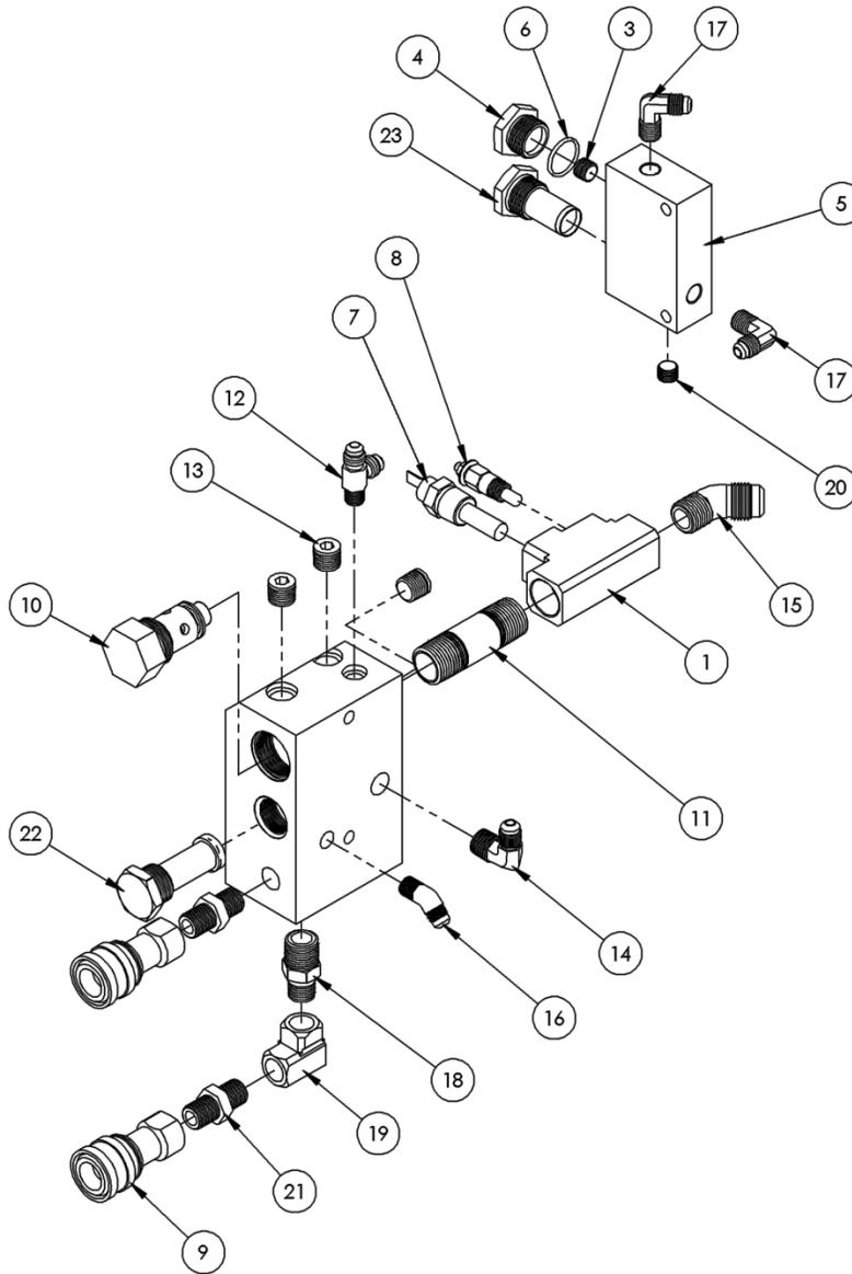
**69-249, ASSY, MANIFOLD BLOCK & BYPASS MANIFOLD, 12 - 23**
