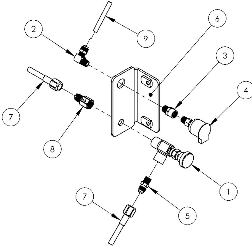
**69-427, ASSEMBLY, OIL CUP AND BYPASS VALVE**
