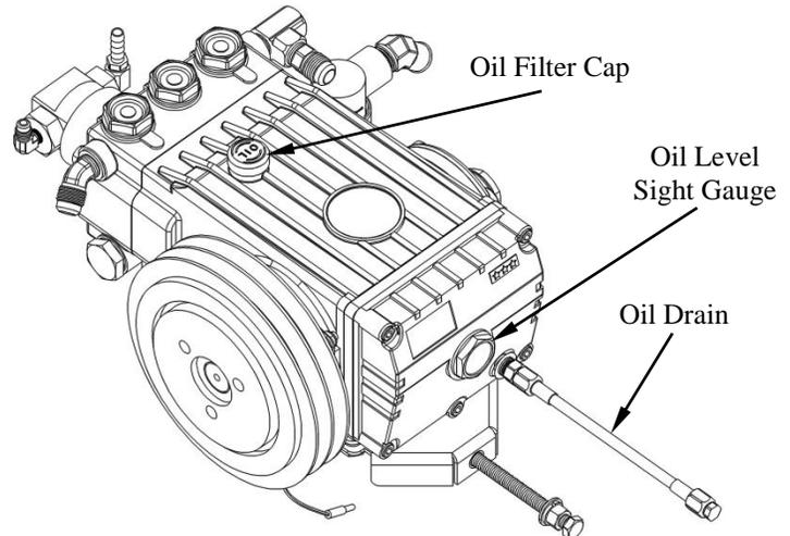
2. After the first **50 hours** of operation, change the crankcase oil Industrial Pump Oil, (Part # 13-030). Change the crankcase oil every **500 hours** thereafter.
