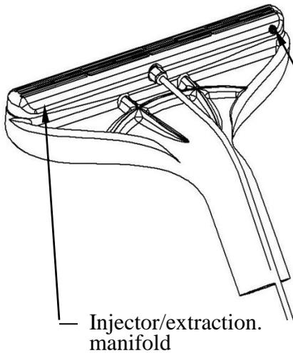
Purge valve. To flush out or debris from injector, loosen purge valve and allow solution to flow at full force.
