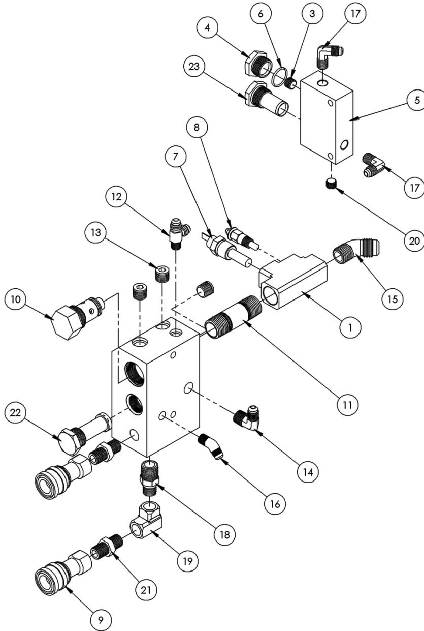
**69-249, ASSY, MANIFOLD BLOCK & BYPASS MANIFOLD, 1 - 11**
